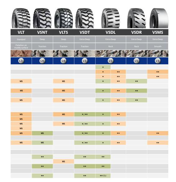
**Star Rating** ( $\star$ ): Indicates the load capacity of a radial tyre at a given inflation pressure.
